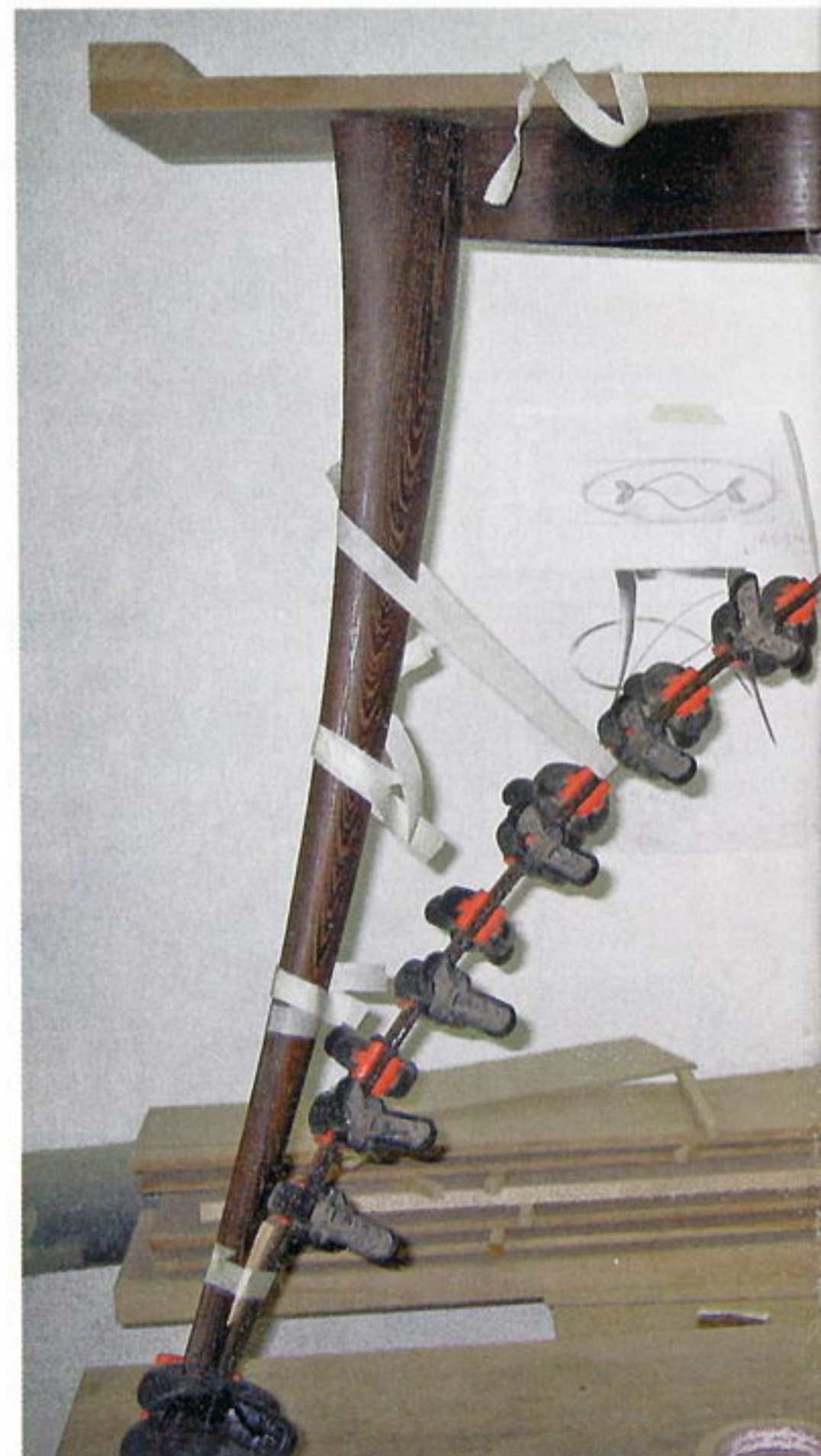
▲ Bulldog cramps are superb for holding laminations together for shaping. In the end Nick chose not to incorporate the 'whizzy wanger' ribbons of wenge as in the original sketch (right)
