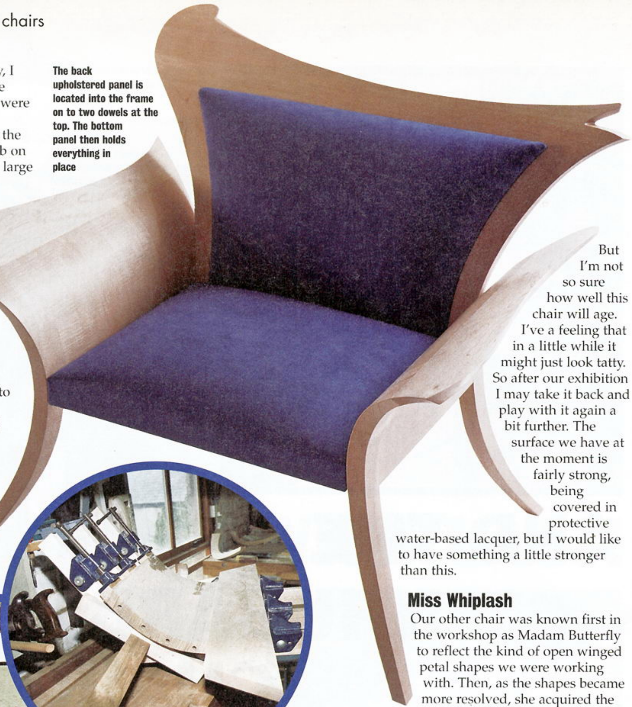
We made our own laminated plywood core for the curved arms. This needed a complicated cramping jig to attach it to the top armrest. Note the dowel holes to register the curved legs
