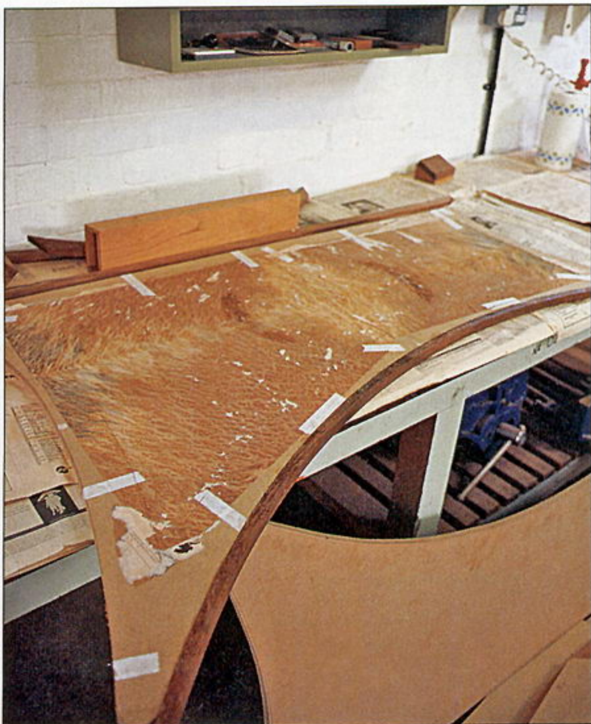
ABOVE: Desk top is veneered with burr panels after a night in the vacuum bag
