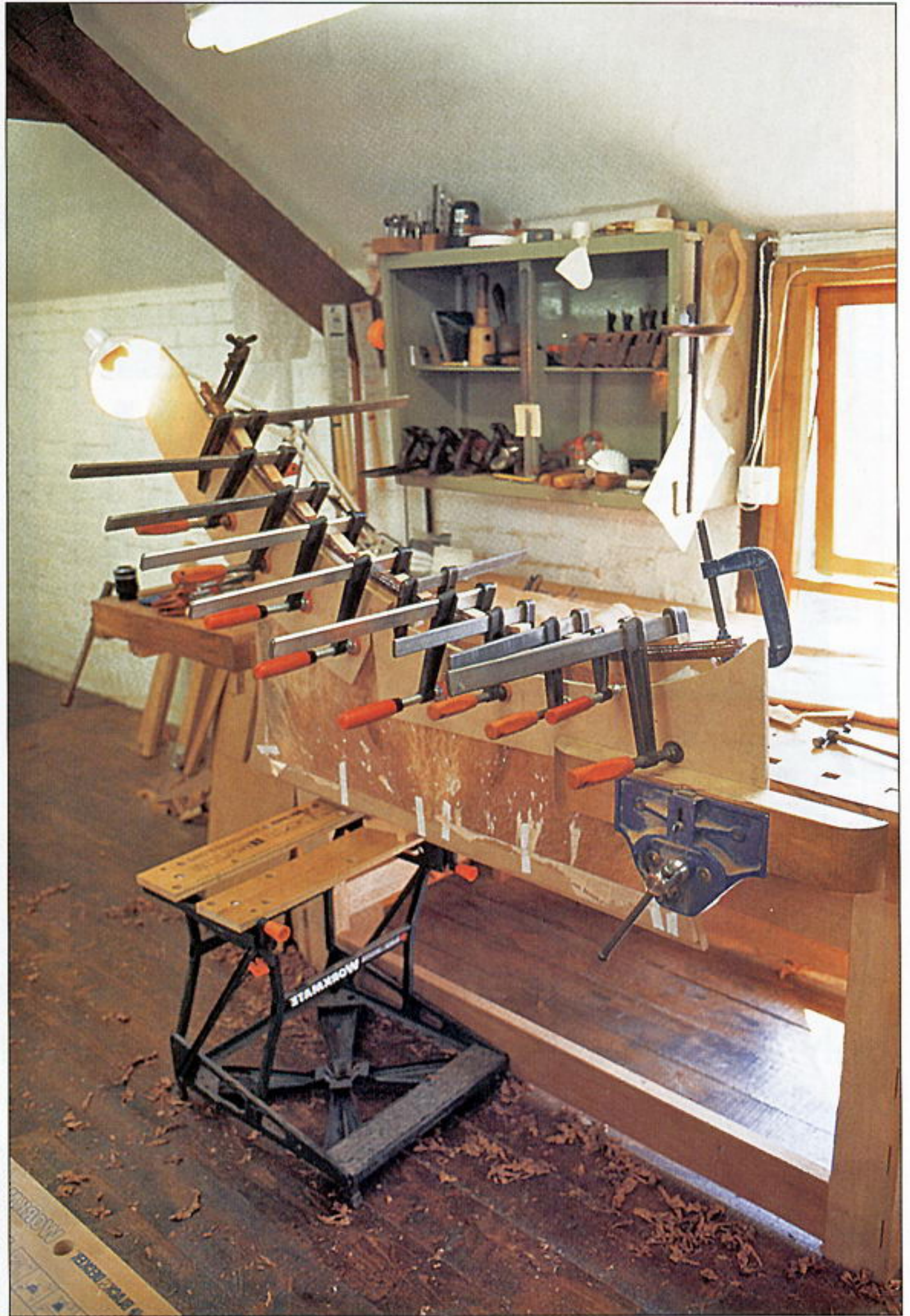
ABOVE AND RIGHT: The lippings for the front and side edges of the desk are laminated; in this case the 2mm thick laminates were bent onto the MDF desk top and held in place with wedges; three laminates were glued up at one time
