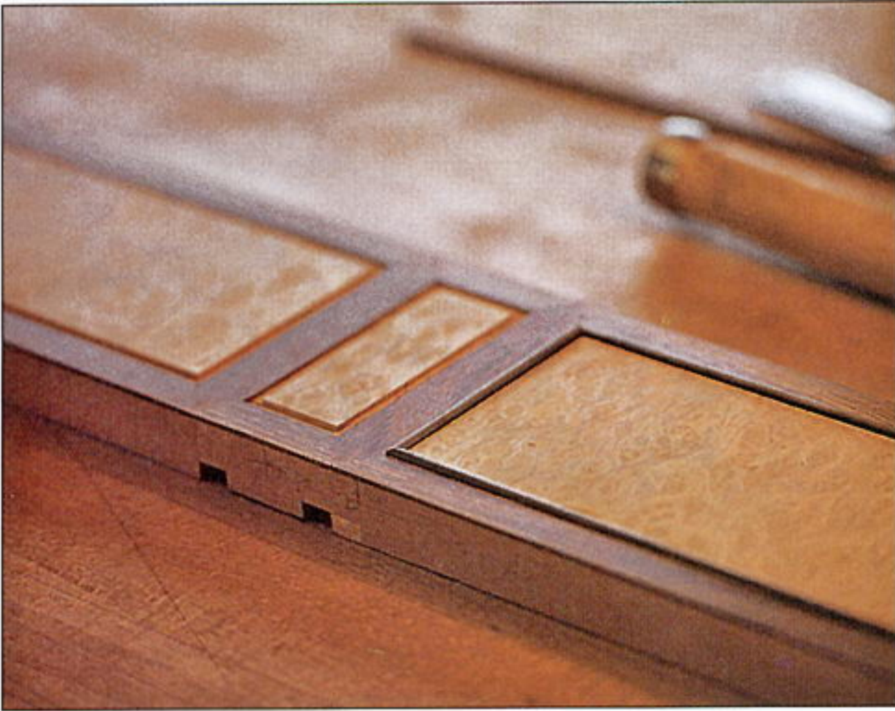
ABOVE: A detail of the desk back panel, showing how slightly raised and domed ebony lines give a light-catching detail
